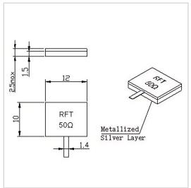
RF Solution offer a wide selection of Leaded Termination for global customers. RFT50-250TM1210 is a Leaded Termination in Frequency Range of DC $\sim$ 3.0 GHz. It is made of high quality materials under a high standard, the Resistance Range of this product is 50  $\Omega$ , Resistance Tolerance is  $\pm 5\%$  and VSWR Max is 1.20. The component has a good working performance and stability, it is ideal for handling a Power of 250 W.
