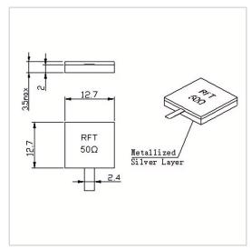
RF Solution offer a wide selection of Leaded Termination for global customers. RFT50-250TM1313B is a Leaded Termination in Frequency Range of DC $\sim$ 10.0 GHz. It is made of high quality materials under a high standard, the Resistance Range of this product is 50  $\Omega$ , Resistance Tolerance is  $\pm 5\%$  and VSWR Max is  $1.20\sim1.30$ . The component has a good working performance and stability, it is ideal for handling a Power of 250 W.
