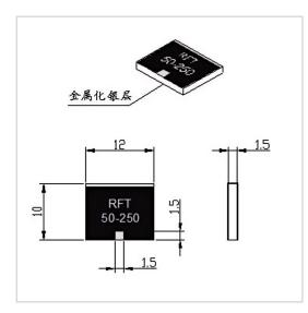
RF Solution offer a wide selection of Chip Termination for global customers. RFT50-250WT1210 is a Chip Termination in Frequency Range of DC $\sim$ 3.0 GHz. It is made of high quality materials under a high standard, the Resistance Range of this product is 50  $\Omega$ , Resistance Tolerance is  $\pm 5\%$  and VSWR Max is 1.20. The component has a good working performance and stability, it is ideal for handling a Power of 250 W.
