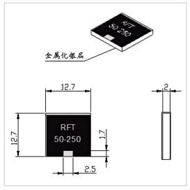
RF Solution offer a wide selection of Chip Termination for global customers. RFT50-250WT1313B is a Chip Termination in Frequency Range of DC~10.0 GHz. It is made of high quality materials under a high standard, the Resistance Range of this product is 50  $\Omega$ , Resistance Tolerance is  $\pm 5\%$  and VSWR Max is 1.20~1.30. The component has a good working performance and stability, it is ideal for handling a Power of 250 W.
