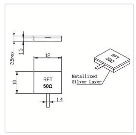
RF Solution offer a wide selection of Leaded Termination for global customers. RFT50-300TM1210 is a Leaded Termination in Frequency Range of DC $\sim$ 3.0 GHz. It is made of high quality materials under a high standard, the Resistance Range of this product is 50  $\Omega$ , Resistance Tolerance is  $\pm 5\%$  and VSWR Max is  $1.20\sim1.30$ . The component has a good working performance and stability, it is ideal for handling a Power of 300 W.
