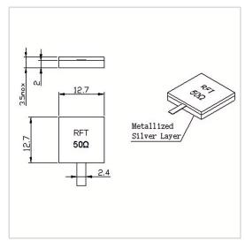
RF Solution offer a wide selection of Leaded Termination for global customers. RFT50-300TM1313B is a Leaded Termination in Frequency Range of DC~10.0 GHz. It is made of high quality materials under a high standard, the Resistance Range of this product is 50  $\Omega$ , Resistance Tolerance is  $\pm 5\%$  and VSWR Max is  $1.20\sim1.30$ . The component has a good working performance and stability, it is ideal for handling a Power of 300 W.
