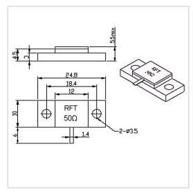
RF Solution offer a wide selection of Flanged Termination for global customers. RFT50-300TM2510 is a Flanged Termination in Frequency Range of DC $\sim$ 3.0 GHz. It is made of high quality materials under a high standard, the Resistance Range of this product is 50  $\Omega$ , Resistance Tolerance is  $\pm 5\%$  and VSWR Max is 1.20. The component has a good working performance and stability, it is ideal for handling a Power of 300 W.
