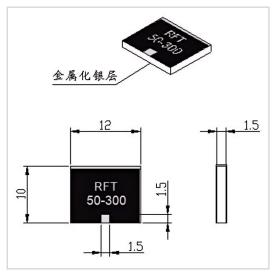
RF Solution offer a wide selection of Chip Termination for global customers. RFT50-300WT1210 is a Chip Termination in Frequency Range of DC~3.0 GHz. It is made of high quality materials under a high standard, the Resistance Range of this product is 50  $\Omega$ , Resistance Tolerance is  $\pm 5\%$  and VSWR Max is 1.20. The component has a good working performance and stability, it is ideal for handling a Power of 300 W.
