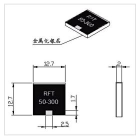
RF Solution offer a wide selection of Chip Termination for global customers. RFT50-300WT1313B is a Chip Termination in Frequency Range of DC $\sim$ 10.0 GHz. It is made of high quality materials under a high standard, the Resistance Range of this product is 50  $\Omega$ , Resistance Tolerance is  $\pm 5\%$  and VSWR Max is  $1.20\sim1.30$ . The component has a good working performance and stability, it is ideal for handling a Power of 300 W.
