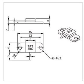
RF Solution offer a wide selection of Flanged Termination for global customers. RFT50-30TM1606 is a Flanged Termination in Frequency Range of DC $\sim$ 6.0 GHz. It is made of high quality materials under a high standard, the Resistance Range of this product is 50  $\Omega$ , Resistance Tolerance is  $\pm 5\%$  and VSWR Max is 1.25. The component has a good working performance and stability, it is ideal for handling a Power of 30 W.
