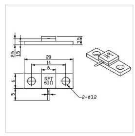
RF Solution offer a wide selection of Flanged Termination for global customers. RFT50-30TM2006 is a Flanged Termination in Frequency Range of DC $\sim$ 6.0 GHz. It is made of high quality materials under a high standard, the Resistance Range of this product is 50  $\Omega$ , Resistance Tolerance is  $\pm 5\%$  and VSWR Max is 1.25. The component has a good working performance and stability, it is ideal for handling a Power of 30 W.
