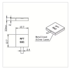
RF Solution offer a wide selection of Leaded Termination for global customers. RFT50-400TM1313 is a Leaded Termination in Frequency Range of DC~2.0 GHz. It is made of high quality materials under a high standard, the Resistance Range of this product is 50  $\Omega$ , Resistance Tolerance is  $\pm 5\%$  and VSWR Max is 1.20~1.30. The component has a good working performance and stability, it is ideal for handling a Power of 400 W.
