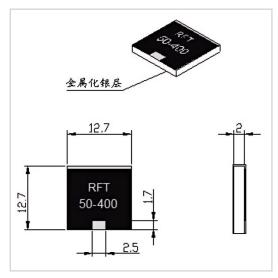
RF Solution offer a wide selection of Chip Termination for global customers. RFT50-400WT1313 is a Chip Termination in Frequency Range of DC $\sim$ 2.0 GHz. It is made of high quality materials under a high standard, the Resistance Range of this product is 50  $\Omega$ , Resistance Tolerance is  $\pm 5\%$  and VSWR Max is 1.20. The component has a good working performance and stability, it is ideal for handling a Power of 400 W.
