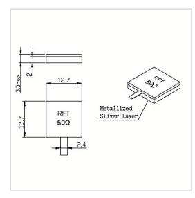
RF Solution offer a wide selection of Leaded Termination for global customers. RFT50-500TM1313 is a Leaded Termination in Frequency Range of DC~2.0 GHz. It is made of high quality materials under a high standard, the Resistance Range of this product is 50  $\Omega$ , Resistance Tolerance is  $\pm 5\%$  and VSWR Max is 1.20. The component has a good working performance and stability, it is ideal for handling a Power of 500 W.
