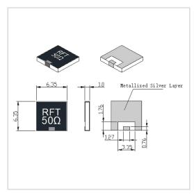
RF Solution offer a wide selection of Chip Termination for global customers. RFT50-60CT6363 is a Chip Termination in Frequency Range of DC $\sim$ 5.0 GHz. It is made of high quality materials under a high standard, the Resistance Range of this product is 50  $\Omega$ , Resistance Tolerance is  $\pm 5\%$  and VSWR Max is  $1.20\sim1.25$ . The component has a good working performance and stability, it is ideal for handling a Power of 60 W.
