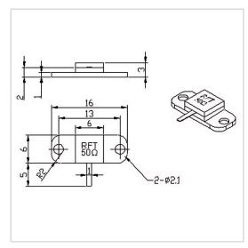
RF Solution offer a wide selection of Flanged Termination for global customers. RFT50-60TM1606 is a Flanged Termination in Frequency Range of DC $\sim$ 6.0 GHz. It is made of high quality materials under a high standard, the Resistance Range of this product is 50  $\Omega$ , Resistance Tolerance is  $\pm 5\%$  and VSWR Max is 1.25. The component has a good working performance and stability, it is ideal for handling a Power of 60 W.
