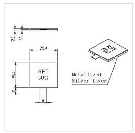
RF Solution offer a wide selection of Leaded Termination for global customers. RFT50-800TM2525 is a Leaded Termination in Frequency Range of DC~8.0 GHz. It is made of high quality materials under a high standard, the Resistance Range of this product is 50  $\Omega$ , Resistance Tolerance is  $\pm 5\%$  and VSWR Max is 1.20. The component has a good working performance and stability, it is ideal for handling a Power of 800 W.
