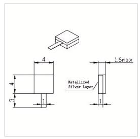
RF Solution offer a wide selection of Leaded Termination for global customers. RFT50A-05TM0404 is a Leaded Termination in Frequency Range of DC $\sim$ 6.0 GHz. It is made of high quality materials under a high standard, the Resistance Range of this product is 50  $\Omega$ , Resistance Tolerance is  $\pm 5\%$  and VSWR Max is 1.20. The component has a good working performance and stability, it is ideal for handling a Power of 5 W.
