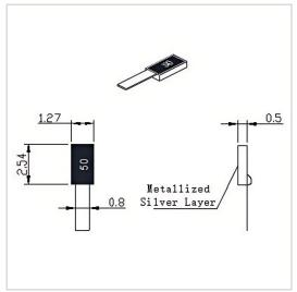
RF Solution offer a wide selection of Leaded Termination for global customers. RFT50N-05TJ1225 is a Leaded Termination in Frequency Range of DC $\sim$ 6.0 GHz. It is made of high quality materials under a high standard, the Resistance Range of this product is 50  $\Omega$ , Resistance Tolerance is  $\pm 5\%$  and VSWR Max is  $1.20\sim1.30$ . The component has a good working performance and stability, it is ideal for handling a Power of 5 W.
