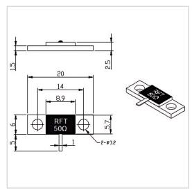
RF Solution offer a wide selection of Flanged Termination for global customers. RFT50N-100TJ2006B is a Flanged Termination in Frequency Range of DC $\sim$ 6.0 GHz. It is made of high quality materials under a high standard, the Resistance Range of this product is 50  $\Omega$ , Resistance Tolerance is  $\pm 5\%$  and VSWR Max is 1.20. The component has a good working performance and stability, it is ideal for handling a Power of 100 W.
