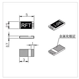
RF Solution offer a wide selection of Chip Termination for global customers. RFT50N-10CT2550 is a Chip Termination in Frequency Range of DC $\sim$ 6.0 GHz. It is made of high quality materials under a high standard, the Resistance Range of this product is 50  $\Omega$ , Resistance Tolerance is  $\pm 5\%$  and VSWR Max is 1.20. The component has a good working performance and stability, it is ideal for handling a Power of 10 W.
