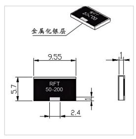
RF Solution offer a wide selection of Chip Termination for global customers. RFT50N-200WT9557 is a Chip Termination in Frequency Range of DC $\sim$ 3.0 GHz. It is made of high quality materials under a high standard, the Resistance Range of this product is 50  $\Omega$ , Resistance Tolerance is  $\pm 5\%$  and VSWR Max is 1.25. The component has a good working performance and stability, it is ideal for handling a Power of 200 W.
