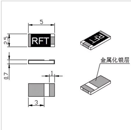
RF Solution offer a wide selection of Chip Termination for global customers. RFT50N-20CT2550 is a Chip Termination in Frequency Range of DC~6.0 GHz. It is made of high quality materials under a high standard, the Resistance Range of this product is 50  $\Omega$ , Resistance Tolerance is  $\pm 5\%$  and VSWR Max is 1.20. The component has a good working performance and stability, it is ideal for handling a Power of 20 W.
