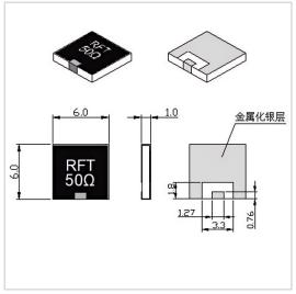
RF Solution offer a wide selection of Chip Termination for global customers. RFT50N-60CT0606 is a Chip Termination in Frequency Range of DC $\sim$ 6.0 GHz. It is made of high quality materials under a high standard, the Resistance Range of this product is 50  $\Omega$ , Resistance Tolerance is  $\pm 5\%$  and VSWR Max is  $1.20\sim1.30$ . The component has a good working performance and stability, it is ideal for handling a Power of 60 W.
