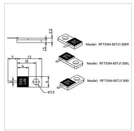
RF Solution offer a wide selection of Flanged Termination for global customers. RFT50N-60TJ1306 is a Flanged Termination in Frequency Range of DC $\sim$ 6.0 GHz. It is made of high quality materials under a high standard, the Resistance Range of this product is 50  $\Omega$ , Resistance Tolerance is  $\pm 5\%$  and VSWR Max is 1.25. The component has a good working performance and stability, it is ideal for handling a Power of 60 W.
