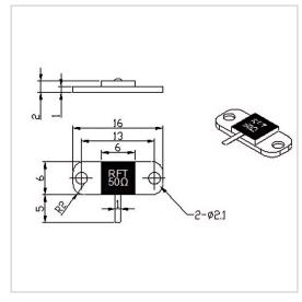
RF Solution offer a wide selection of Flanged Termination for global customers. RFT50N-60TJ1606 is a Flanged Termination in Frequency Range of DC $\sim$ 6.0 GHz. It is made of high quality materials under a high standard, the Resistance Range of this product is 50  $\Omega$ , Resistance Tolerance is  $\pm 5\%$  and VSWR Max is 1.25. The component has a good working performance and stability, it is ideal for handling a Power of 60 W.
