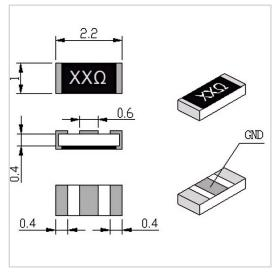
RF Solution offer a wide selection of Chip Resistor for global customers. RFTXX-05CR1022C is a Chip Resistor in Resistance Range of XX  $\Omega$  (10~3000 $\Omega$  Customizable). It is made of high quality materials under a high standard, the Resistance Tolerance of this product is  $\pm 5\%$ , Substrate Material is BeO and Resistive Element is Thick Film. The component has a good working performance and stability, it is ideal for handling a Power of 5 W.
