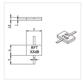
RF Solution offer a wide selection of Leaded Attenuator for global customers. RFTXX-100AM0906-6 is a Leaded Attenuator in Frequency Range of DC $\sim$ 6.0 GHz. It is made of high quality materials under a high standard, the Attenuation Value of this product is @01-10 dB@14,15,20 dB@25,30 dB, Attenuation Tolerance is  $@\pm0.6 dB@\pm0.8 dB@\pm1.0dB$  and VSWR Max is 1.25. The component has a good working performance and stability, it is ideal for handling a Rated Power of 100 W.
