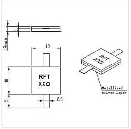
RF Solution offer a wide selection of Leaded Resistor for global customers. RFTXX-100RM1010 is a Leaded Resistor in Capacitance of 5.6 PF@50 $\Omega$ . It is made of high quality materials under a high standard, the Resistance Range of this product is XX  $\Omega$  (10-1500 $\Omega$  Customizable), Resistance Tolerance is  $\pm 5\%$  and Temperature Coefficient Max is 150 ppm/°C. The component has a good working performance and stability, it is ideal for handling a Power of 100 W.
