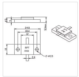
RF Solution offer a wide selection of Flanged Resistor for global customers. RFTXX-100RM2510 is a Flanged Resistor in Capacitance of 5.6 PF@100 $\Omega$ . It is made of high quality materials under a high standard, the Resistance of this product is XX  $\Omega$  (10~1000 $\Omega$  Customizable), Resistance Tolerance is  $\pm 5\%$  and Temperature Coefficient Max is 150 ppm/°C. The component has a good working performance and stability, it is ideal for handling a Power of 100 W.
