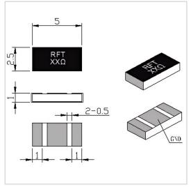
RF Solution offer a wide selection of Chip Resistor for global customers. RFTXX-10CR2550C is a Chip Resistor in Resistance Range of XX  $\Omega$  (10~3000 $\Omega$  Customizable). It is made of high quality materials under a high standard, the Resistance Tolerance of this product is  $\pm 5\%$ , Substrate Material is BeO and Resistive Element is Thick Film. The component has a good working performance and stability, it is ideal for handling a Power of 10 W.
