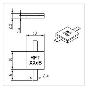
RF Solution offer a wide selection of Leaded Attenuator for global customers. RFTXX-150AM1010-3 is a Leaded Attenuator in Frequency Range of DC~3.0 GHz. It is made of high quality materials under a high standard, the Attenuation Value of this product is 2522627 dB30 dB, Attenuation Tolerance is +0.8/-1.5 dB40 dB and VSWR Max is 1.25. The component has a good working performance and stability, it is ideal for handling a Rated Power of 150 W.
