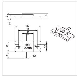
RF Solution offer a wide selection of Flanged Attenuator for global customers. RFTXX-150AM2310-3 is a Flanged Attenuator in Frequency Range of DC~3.0 GHz. It is made of high quality materials under a high standard, the Attenuation Value of this product is \$\mathbb{Q}\$25,26,27 dB@30 dB, Attenuation Tolerance is \$\mathbb{Q}\$+0.8/-1.5 dB@±1.0 dB and VSWR Max is 1.25. The component has a good working performance and stability, it is ideal for handling a Rated Power of 150 W.
