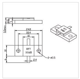
RF Solution offer a wide selection of Flanged Attenuator for global customers. RFTXX-150AM2510-3 is a Flanged Attenuator in Frequency Range of DC $\sim$ 3.0 GHz. It is made of high quality materials under a high standard, the Attenuation Value of this product is @25,26,27 dB@30 dB, Attenuation Tolerance is @+0.8/-1.5 dB@ $\pm1.0$  dB and VSWR Max is 1.25. The component has a good working performance and stability, it is ideal for handling a Rated Power of 150 W.
