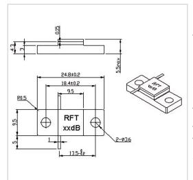
RF Solution offer a wide selection of Flanged Attenuator for global customers. RFTXX-150AM2595B-3 is a Flanged Attenuator in Frequency Range of DC~3.0 GHz. It is made of high quality materials under a high standard, the Attenuation Value of this product is 12 dB = 30 dB, Attenuation Tolerance is  $\pm 0.7 \text{ dB} = \pm 1.0 \text{ dB}$  and VSWR Max is 1.25. The component has a good working performance and stability, it is ideal for handling a Rated Power of 150 W.
