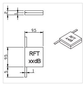
RF Solution offer a wide selection of Leaded Attenuator for global customers. RFTXX-150AM9595B-3 is a Leaded Attenuator in Frequency Range of DC~3.0 GHz. It is made of high quality materials under a high standard, the Attenuation Value of this product is \$\mathbb{U}\$12 dB\$230 dB, Attenuation Tolerance is \$\mathbb{U}\$±0.7 dB\$2±1.0 dB and VSWR Max is 1.25. The component has a good working performance and stability, it is ideal for handling a Rated Power of 150 W.
