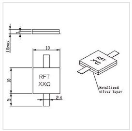
RF Solution offer a wide selection of Leaded Resistor for global customers. RFTXX-150RM1010 is a Leaded Resistor in Capacitance of 5.6 PF@50 $\Omega$ . It is made of high quality materials under a high standard, the Resistance Range of this product is XX  $\Omega$  (10-1500 $\Omega$  Customizable), Resistance Tolerance is  $\pm 5\%$  and Temperature Coefficient Max is 150 ppm/°C. The component has a good working performance and stability, it is ideal for handling a Power of 150 W.
