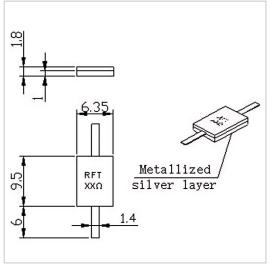
RF Solution offer a wide selection of Leaded Resistor for global customers. RFTXX-150RM6395 is a Leaded Resistor in Capacitance of 3.9 PF@50 $\Omega$ . It is made of high quality materials under a high standard, the Resistance Range of this product is XX  $\Omega$  (10-1500 $\Omega$  Customizable), Resistance Tolerance is  $\pm 5\%$  and Temperature Coefficient Max is 150 ppm/°C. The component has a good working performance and stability, it is ideal for handling a Power of 150 W.
