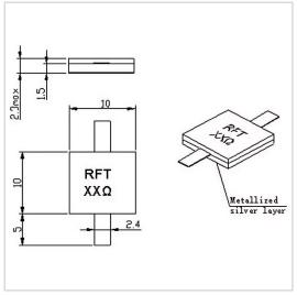
RF Solution offer a wide selection of Leaded Resistor for global customers. RFTXX-200RM1010B is a Leaded Resistor in Capacitance of 4.0 PF@100 $\Omega$ . It is made of high quality materials under a high standard, the Resistance Range of this product is XX  $\Omega$  (10-1500 $\Omega$  Customizable), Resistance Tolerance is  $\pm 5\%$  and Temperature Coefficient Max is 150 ppm/°C. The component has a good working performance and stability, it is ideal for handling a Power of 200 W.
