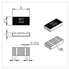
RF Solution offer a wide selection of Chip Resistor for global customers. RFTXX-20CR2550C is a Chip Resistor in Resistance Range of XX  $\Omega$  ( $10\sim3000\Omega$  Customizable). It is made of high quality materials under a high standard, the Resistance Tolerance of this product is  $\pm5\%$ , Substrate Material is BeO and Resistive Element is Thick Film. The component has a good working performance and stability, it is ideal for handling a Power of 20 W.
