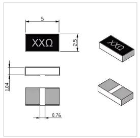
RF Solution offer a wide selection of Chip Resistor for global customers. RFTXX-20CR2550TA is a Chip Resistor in Resistance Range of XX  $\Omega$  ( $10\sim3000\Omega$  Customizable). It is made of high quality materials under a high standard, the Resistance Tolerance of this product is  $\pm5\%$ , Substrate Material is BeO and Resistive Element is Thick Film. The component has a good working performance and stability, it is ideal for handling a Power of 20 W.
