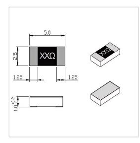
RF Solution offer a wide selection of Chip Resistor for global customers. RFTXX-20CR2550W is a Chip Resistor in Resistance Range of XX  $\Omega$  ( $10\sim3000\Omega$  Customizable). It is made of high quality materials under a high standard, the Resistance Tolerance of this product is  $\pm5\%$ , Substrate Material is BeO and Resistive Element is Thick Film. The component has a good working performance and stability, it is ideal for handling a Power of 20 W.
