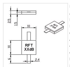
RF Solution offer a wide selection of Leaded Attenuator for global customers. RFTXX-250AM1010-1.5 is a Leaded Attenuator in Frequency Range of DC~1.5 GHz. It is made of high quality materials under a high standard, the Attenuation Value of this product is 01-03 dB20dB30 dB, Attenuation Tolerance is  $0\pm0.6$  dB $2\pm0.8$ dB $3\pm1.0$  dB and VSWR Max is 1.25. The component has a good working performance and stability, it is ideal for handling a Rated Power of 250 W.
