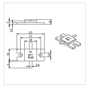
RF Solution offer a wide selection of Flanged Attenuator for global customers. RFTXX-250AM2310-1.5 is a Flanged Attenuator in Frequency Range of DC $\sim$ 1.5 GHz. It is made of high quality materials under a high standard, the Attenuation Value of this product is 01-03 dB20 dB30 dB, Attenuation Tolerance is  $0\pm0.6$  dB $2\pm0.8$  dB $3\pm1.0$  dB and VSWR Max is 1.25. The component has a good working performance and stability, it is ideal for handling a Rated Power of 250 W.
