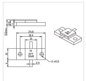
RF Solution offer a wide selection of Flanged Attenuator for global customers. RFTXX-250AM2510-1.5 is a Flanged Attenuator in Frequency Range of DC~1.5 GHz. It is made of high quality materials under a high standard, the Attenuation Value of this product is 01-03 dB220dB330 dB, Attenuation Tolerance is  $0\pm0.6$  dB $2\pm0.8$ dB $3\pm1.0$  dB and VSWR Max is 1.25. The component has a good working performance and stability, it is ideal for handling a Rated Power of 250 W.
