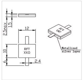
RF Solution offer a wide selection of Leaded Resistor for global customers. RFTXX-250RM1210 is a Leaded Resistor in Capacitance of 5.0 PF@100 $\Omega$ . It is made of high quality materials under a high standard, the Resistance Range of this product is XX  $\Omega$  (10-1000 $\Omega$  Customizable), Resistance Tolerance is  $\pm 5\%$  and Temperature Coefficient Max is 150 ppm/°C. The component has a good working performance and stability, it is ideal for handling a Power of 250 W.
