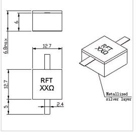
RF Solution offer a wide selection of Leaded Resistor for global customers. RFTXX-250RM1313K is a Leaded Resistor in Capacitance of 2.0 PF@100 $\Omega$ . It is made of high quality materials under a high standard, the Resistance Range of this product is XX  $\Omega$  (10-1000 $\Omega$  Customizable), Resistance Tolerance is  $\pm 5\%$  and Temperature Coefficient Max is 150 ppm/°C. The component has a good working performance and stability, it is ideal for handling a Power of 250 W.
