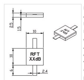
RF Solution offer a wide selection of Leaded Attenuator for global customers. RFTXX-300AM1010-1.5 is a Leaded Attenuator in Frequency Range of DC~1.5 GHz. It is made of high quality materials under a high standard, the Attenuation Value of this product is 01-03 dB230dB, Attenuation Tolerance is  $2\pm0.6$  dB $2\pm1.0$  dB and VSWR Max is 1.25. The component has a good working performance and stability, it is ideal for handling a Rated Power of 300 W.
