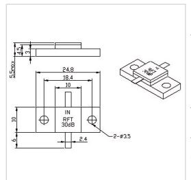
RF Solution offer a wide selection of Flanged Attenuator for global customers. RFTXX-300AM2510-1.5 is a Flanged Attenuator in Frequency Range of DC~1.5 GHz. It is made of high quality materials under a high standard, the Attenuation Value of this product is 01-03 dB230dB, Attenuation Tolerance is  $2\pm0.6$  dB $2\pm1.0$  dB and VSWR Max is 1.25. The component has a good working performance and stability, it is ideal for handling a Rated Power of 250 W.
