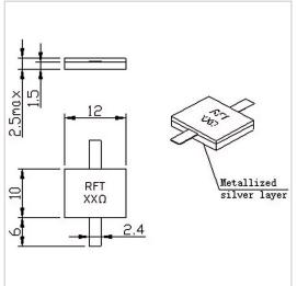
RF Solution offer a wide selection of Leaded Resistor for global customers. RFTXX-300RM1210 is a Leaded Resistor in Capacitance of 5.0 PF@100 $\Omega$ . It is made of high quality materials under a high standard, the Resistance Range of this product is XX  $\Omega$  (10-1000 $\Omega$  Customizable), Resistance Tolerance is  $\pm 5\%$  and Temperature Coefficient Max is 150 ppm/°C. The component has a good working performance and stability, it is ideal for handling a Power of 300 W.
